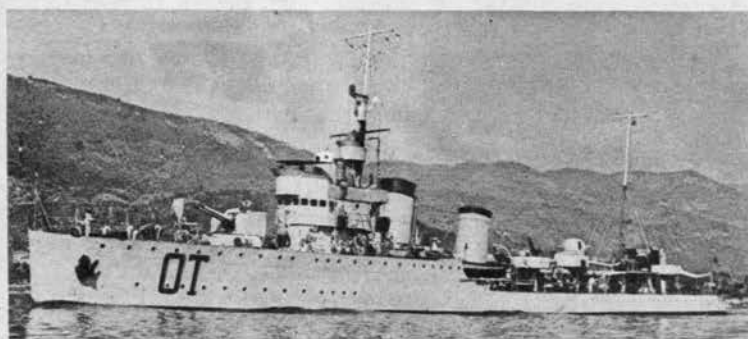
SELLA CLASS typifies old Italian two-stack DD's. Rounded, smooth-surfaced bridge set close to forestack and long forecastle are features.
